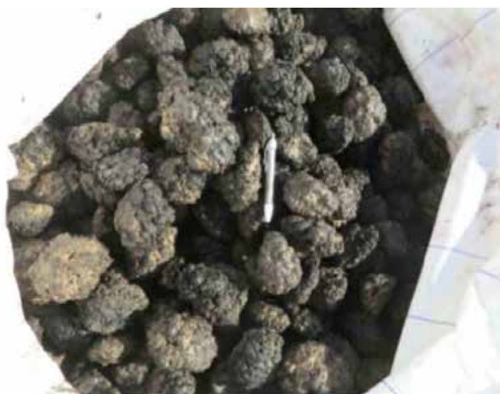
Above: The epibenthic sled used to collect nodules during the 2013 NORI Cruise Below: Polymetallic nodules recovered during the 2013 NORI Cruise Source: Technical Report Summary, AMC Project 321012, 17 March 2021
