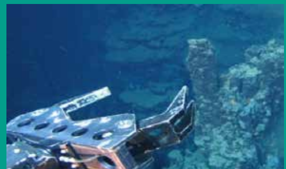
Above: Remote sampling of polymetallic sulphide outcrop at 1700m below sea level
